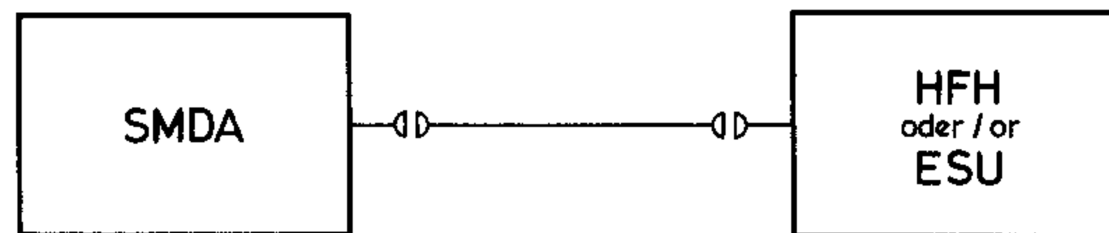
Fig. 3-4 Test setup for harmonics measurement
